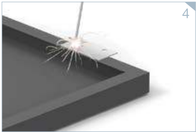
4. Welding the bracket Welding bended panel and bracket(angle)
